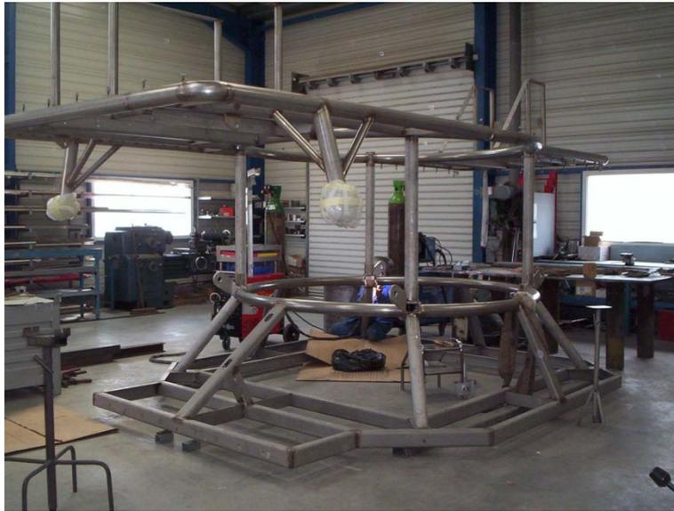
The tubular structure is made of a 88.9mm OD thickness 4 mm Stainless steel pipe.
