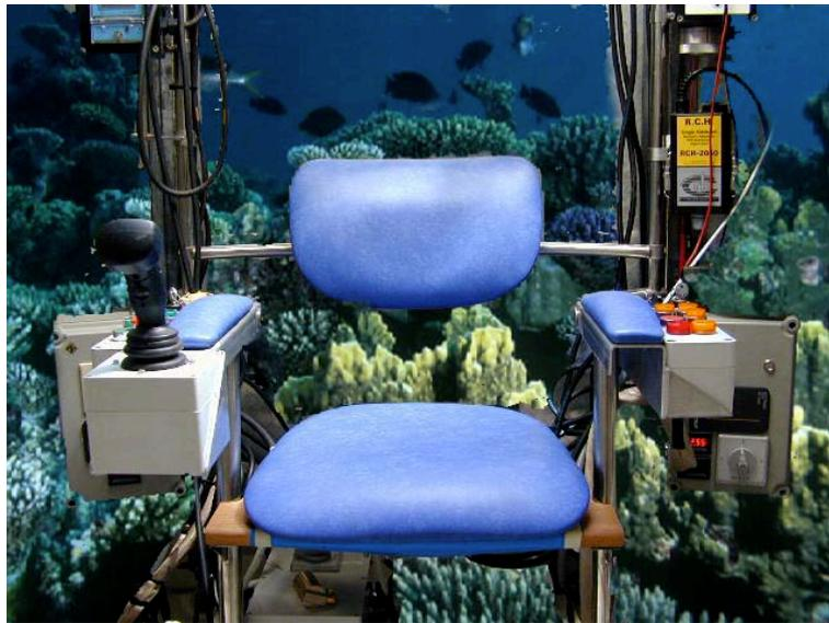
The pilot communicates by mean of VHF radio when on surface and by ultra sonic telephone when underwater (20 W 25 KHz).
