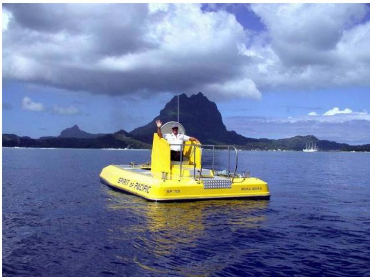
The upper deck is made of fiberglass covered with anti-slip paint and fixed to the pipe frame.
