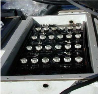
Marine standard lead acid batteries are used in soft fiberglass tanks that are filled with oil and pressure compensated. Hydrogen is captured on the top of each cover of tank. Safety valves open by themselves when hydrogen pressure is above 100mbar.
