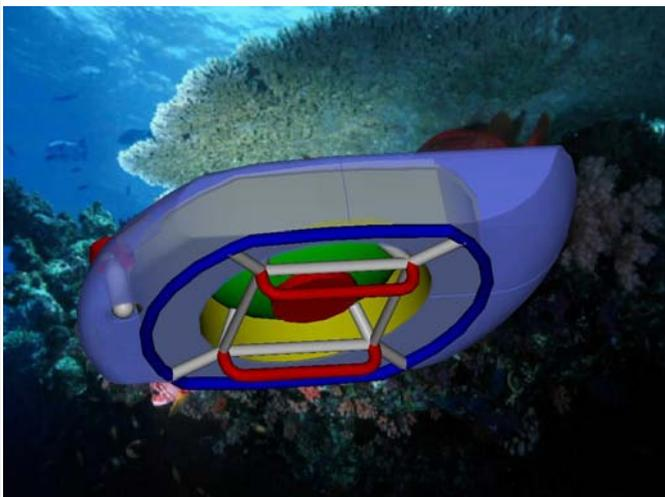
The tubular structure is made of a 88.9mm OD thickness 4 mm steel pipe.
